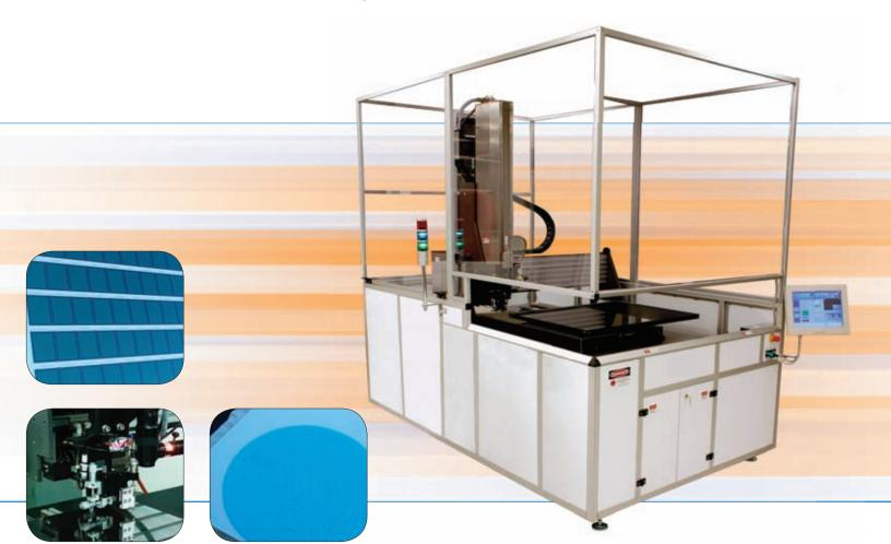
The Fantom G6 Glass Panel Scribing Machine utilizes the latest laser technology for glass scribing and is equipped with an integrated Laser Photonics laser source for the Flat Panel Display Industry.
